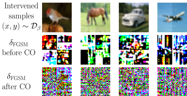
Figure 2: Different samples of the intervened dataset \tilde{\mathcal{D}}_\beta , and FGSM perturbations before and after CO. While prior to CO perturbations focus on the injected features, after CO they become noisy.
