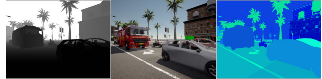
Figure 3. Multimodality is well supported in CARLA, while it may be very difficult to obtain synced data from different sensors in a real-world dataset. From left to right, the depth image, the RGB image and the ground truth (i.e., instance segmentation masks) provide well aligned data for research that explores the relations among different modalities.
