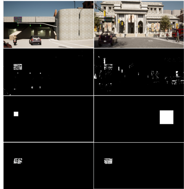
Figure 7. Generalization of adversarial patch defense using physical constraints (Feng et al., 2022). The left column includes a low resolution RGB image and the visualization after applying the defense, while the right column is a high resolution RGB image with the visualized defenses. The first row shows two adversarial images with an adversarial patch in the top left quadrant. The second row shows masks of pixels with anomalous colors. The third row shows masks in regions with high frequency contents. And the fourth row shows masks in regions with high hue and saturation pixel values. This defense, which was trained on low resolution images, performs well on the left column images as it is able to identify the patch location. However, it does not generalize well on high resolution images as shown in the right column where the patch is located at wrong position or false positives occur.
