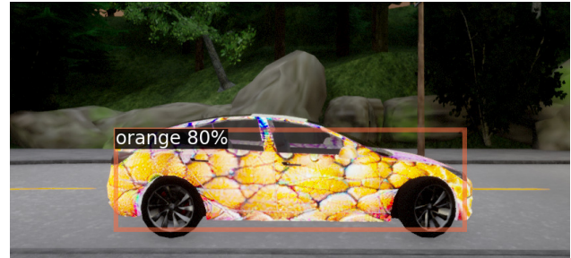
Figure 8. Validation of a ShapeShifter attack in CARLA. An adversarial texture is computed and then applied to a Tesla Model 3 car in the simulation. This attack is successful as it causes the vehicle to be misclassified as an orange.
