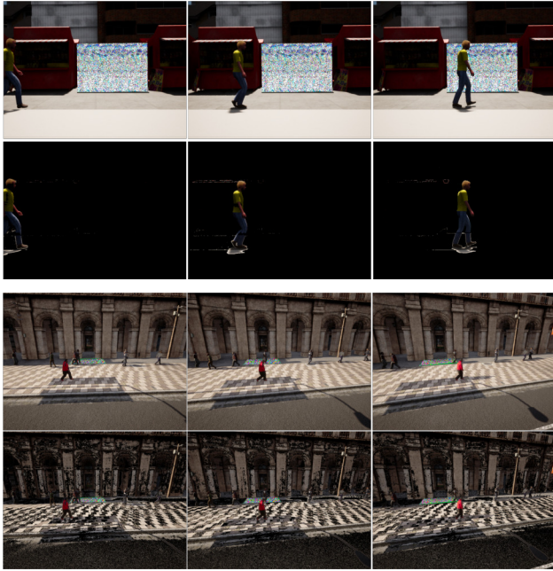
Figure 6. Generalization of the adversarial patch defense using background ablation. Figures at top two rows show that an adversarial attack on a video with a static background, and the defense successfully ablates the adversarial patch. However, as shown by the figures in the bottom two rows, an attack on a tracking video with dynamic background causes the defense fail to ablate the adversarial patch.
