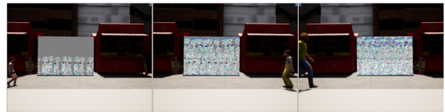
Figure 5. An example of how the simulation tool helps a patch attack generalize better with more object tracking data. The left figure shows that the attack overfits to a single pedestrian tracking video. In the middle figure, the attack improves as it is computed over five tracking videos. The attack shown in the right figure is optimized with ten diverse tracking videos and hence performs the best among the three.
